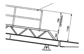
✓ Standard rail guard height is 350 mm in all types oframps. 1100 mm rail guards can be chosen.
